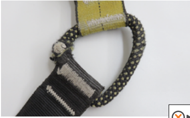
• Damaged attachment point
