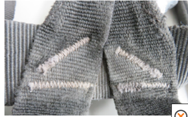
• Damaged safety stitching
