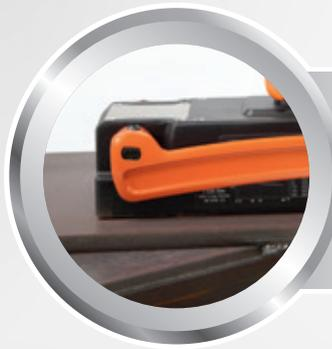
The magnetic field concentrates directly on the material and reduces scattering losses to a minimum.
