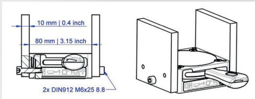
3. Be sure to use the stated torque when screwing.
