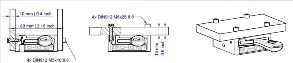
2. Mounting on the magnetic bottom plate made of steel requires at least two screws at any time.
