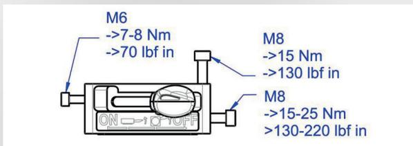
4. Ensure an equal load distribution and introduction to avoid mechanical failure of the magnetic clamp or the mounting materials.
