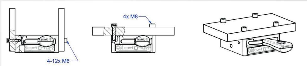
2. Mounting on the magnetic bottom plate made of steel requires at least two screws at any time. (Hardened steel HRC 42)
